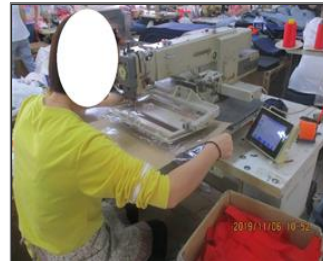
Photo of non-conformity NC No needle guard for computer sewing machine.JPG
