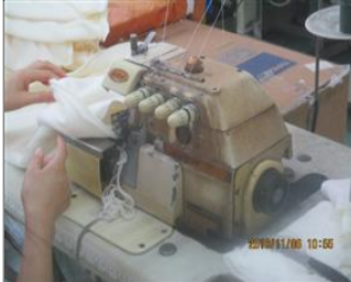
Photo of non-conformity NC No needle guard for locker sewing machine.JPG
