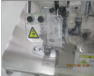
Photo of the inside of the main production hall Needle guard for locker sewing machine.JPG
