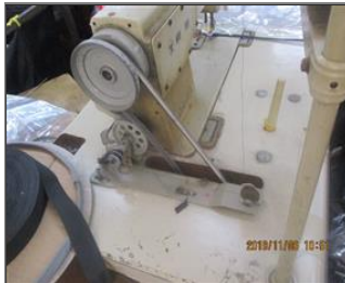
Photo of non-conformity NC No belt guard for sewing machine.JPG
