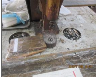
Photo of non-conformity NC No protection equipment for button machine.JPG
